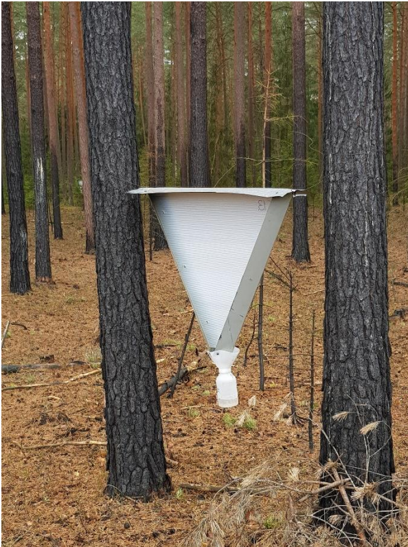
Fig. 5. An IBL2-bis type window trap used to collect beetles in the burnt forest and the control plot (photo J. M. Gutowski).
